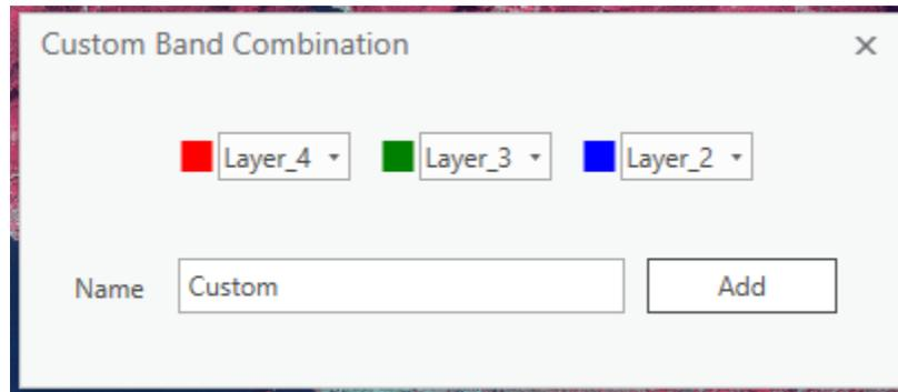
This will produce a standard false color composite. In this image, red areas generally indicated the presence of vegetation, as vegetation is very reflective in the near infrared wavelengths.
